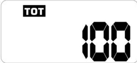
The counter displays the total number of shots fired in the entire service life of the gun, and cannot be reset.
