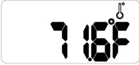
To select the unit of measure for temperature, hold the ON button down for five seconds.
